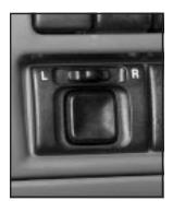
If your vehicle has power mirrors, the selector switch is located on the lower left side of the instrument panel.
